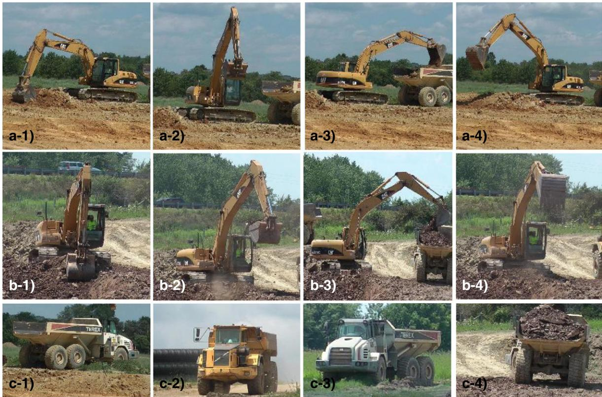
**Fig. 9.** Example frames from video sequences of excavator and truck operations. From left to right in rows (a) and (b): digging, hauling, dumping, and swinging action classes which illustrate tremendous appearance changes because of variability in equipment part arrangement. Row (c) shows the appearance changes due to view point location for a truck (e.g., side view, frontal view).
