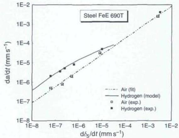
**Figure 20** Crack growth velocity,  $da/dt$ , measured as a function of the applied deformation rate,  $d\delta_5/dt$ , in tests performed in air and in corrosive environment promoting hydrogen embrittlement; the solid curve was obtained from simulation based on a diffusion model (material and environment as in Figure 19) (Dietzel *et al.*, 2005).
