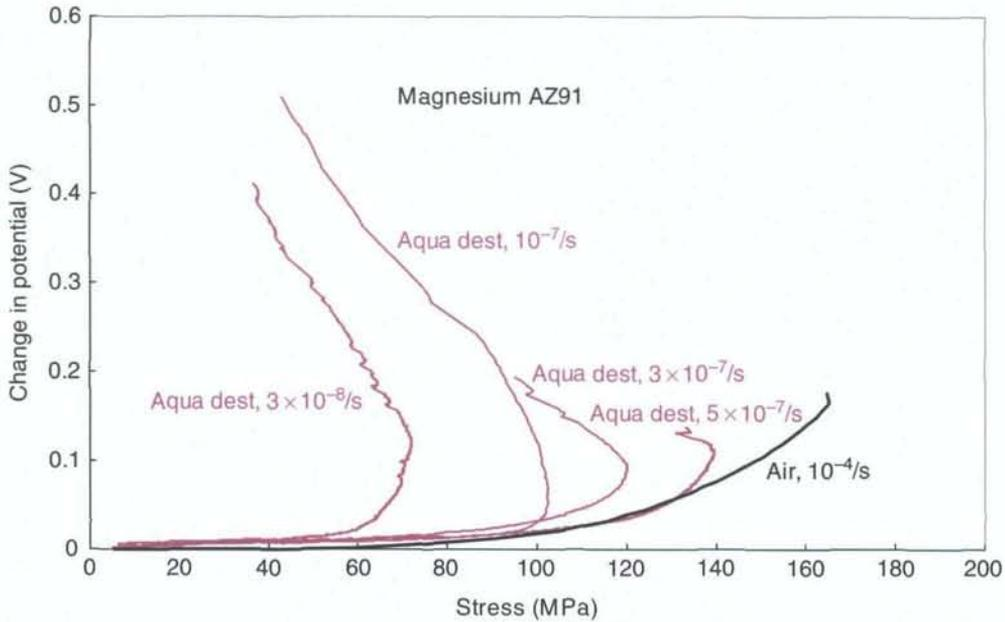
**Figure 10** Potential drop curves for five cylindrical tensile specimens (material: magnesium AZ91) tested in SSRTs in laboratory air and in distilled water.
