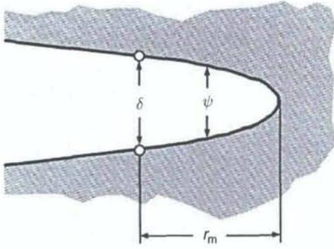
**Figure 14** Definition of the crack-tip opening angle (CTOA),  $\psi$ .
