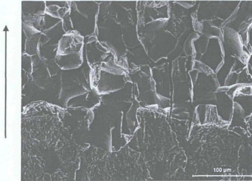
**Figure 5** Scanning electron micrograph showing the transition from a fatigue precrack (lower region) to a stress corrosion crack (upper region) in an austenitic stainless steel (AISI 316H) in 100 ppm Cl<sup>-</sup> solution at 90 °C; the arrow indicates the direction of crack extension (Dietzel, 1999).
