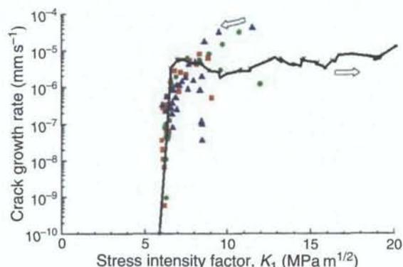
**Figure 8** Comparison of the  $da/dt$  vs  $K$  data of **Figure 6b** (colored symbols) and a  $v$ – $K$  curve (line) determined in a rising displacement test at a compact specimen using the same material/environment combination. The arrows indicate the direction in which the curve is followed in the two different types of test.
