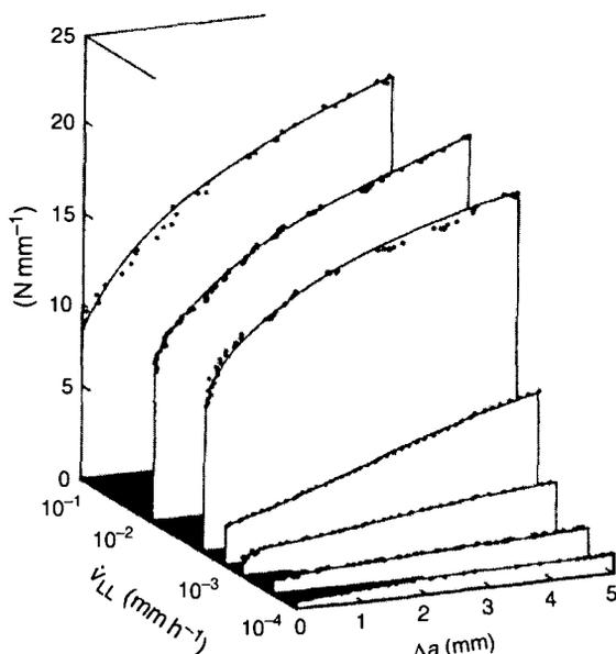
**Figure 13**  $J$ - $R$  curves determined on precracked compact specimens of the aluminum alloy AA 2024 T351 (S-L orientation) in chromated 3.5% NaCl solution using various constant extension rates, measured in the load lines of the specimens (Dietzel, 1991).
