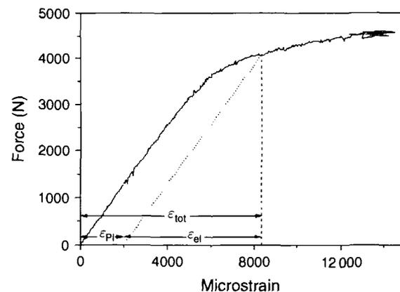
**Figure 2** Illustration showing determination of total strain ( $\epsilon_{tot}$ ) to be applied to achieve 0.2% plastic strain ( $\epsilon_{pl}$ ) in four-point bend testing; the elastic strain is  $\epsilon_{el}$  (Turnbull and Nimmo, 2004).
