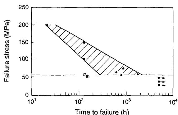
Figure 1 Influence of the initial stress,  $\sigma_{init}$ , on the time to failure,  $t_f$ , measured in constant-load tests on tensile specimens of the high-strength aluminum alloy AA 2024 T351 in a chromated 3.5% sodium chloride solution (Dietzel, 1991).
