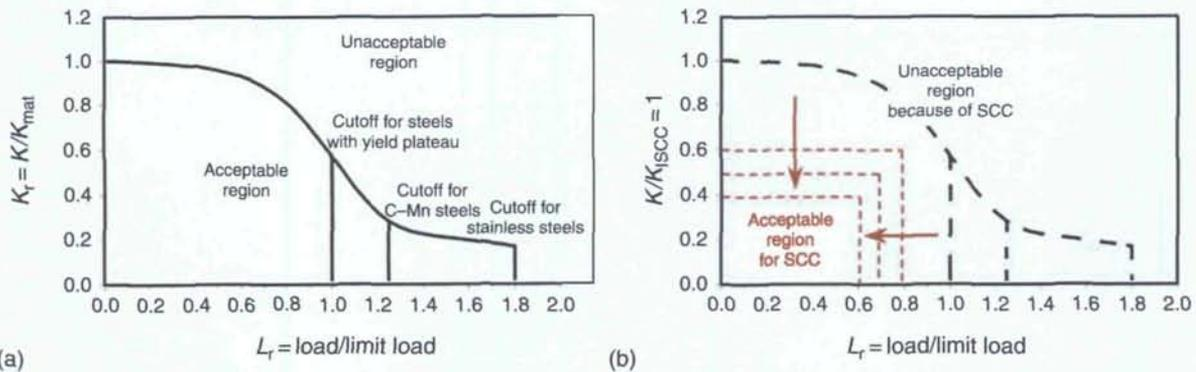
**Figure 18** Schematic presentation illustrating the inclusion of  $K_{I_{SCC}}$  data into a failure assessment diagram (FAD). By substituting the fracture toughness of the material,  $K_{mat}$ , for  $K_{I_{SCC}}$ , and the cutoff line on the stress axis,  $L_r$ , for the SCC threshold stress,  $\sigma_{th}$ , an acceptable region with respect to nongrowing SCCs is defined; this region can be significantly smaller than the original acceptable region as determined from tests in air.
