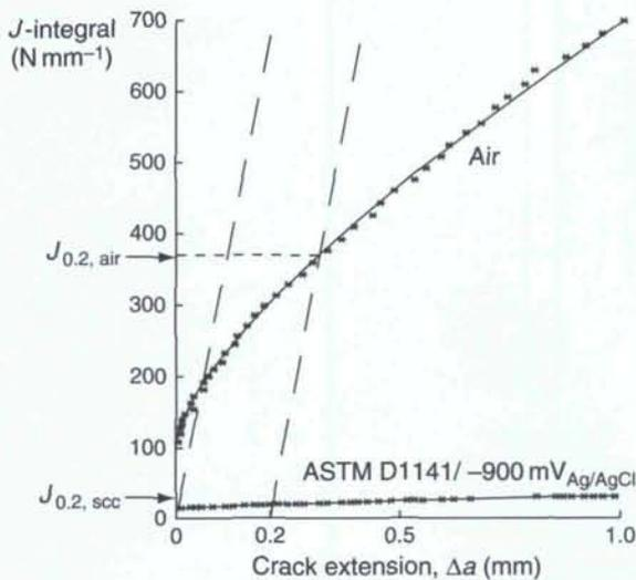
**Figure 19**  $J$ - $R$  curves measured in air and in a corrosive environment promoting the ingress of hydrogen due to cathodic polarization (material: high strength steel, environment ASTM D1141 substitute ocean water) (Dietzel and Schwalbe, 1990).
