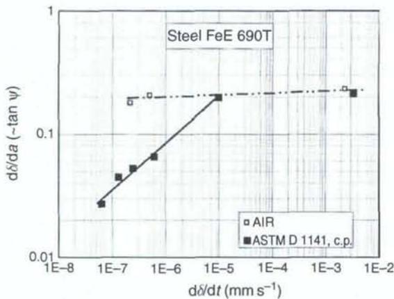
**Figure 15** Values of the tangents of the CTOA,  $\psi$ , determined in rising-displacement tests on compact specimens of a high-strength steel (FeE 690T) subjected to hydrogen embrittlement due to cathodic protection (Dietzel, 1991).
