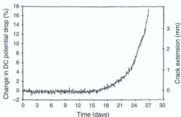
**Figure 7** Crack extension measured in a compact specimen under rising displacement at a rate of  $5.6 \times 10^{-11} \text{ m s}^{-1}$  ( $0.2 \mu\text{m h}^{-1}$ ) in a chromated 3.5% sodium chloride solution (material: aluminum AA 2024 T351); the figure shows the signal obtained using the electrical resistance measurement technique as described in Section 11.03.5.1 (Dietzel, 1991).
