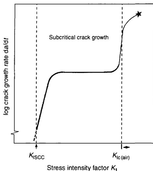
**Figure 4** Effect of the stress intensity factor,  $K_I$ , on the stress corrosion crack growth rate,  $da/dt$  in the region of subcritical crack growth (schematic). After Speidel, M. O. 1971. Current understanding of stress corrosion crack growth in aluminium alloys. In: *The Theory of Stress Corrosion Cracking* (ed. J. C. Scully), pp 289–344. NATO, Brussels.
