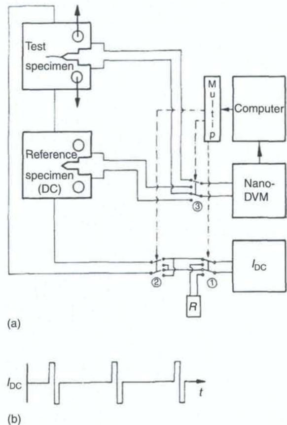
**Figure 11** a, Circuit for DCPD measurement of crack lengths on compact specimens in SCC tests in aqueous environments, using a reference specimen and a pulsed current with switching of polarity; b, pulsed current sent through both the test specimen and the reference specimen. Reproduced with permission from Dietzel, W. and Schwalbe, K.-H. 1986. Monitoring stable crack growth using a combined AC/DC potential drop technique. *Z. Materialprüfung/Materials Testing* 28(11), 368–372.
