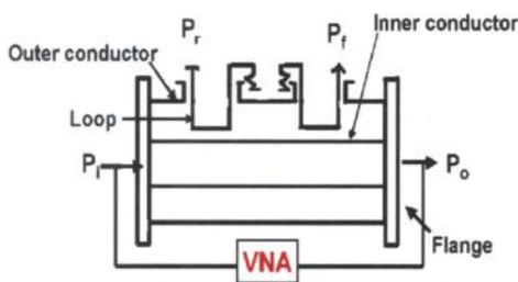
Fig. 3. Schematic of test setup for low power RF testing of coaxial directional coupler.
