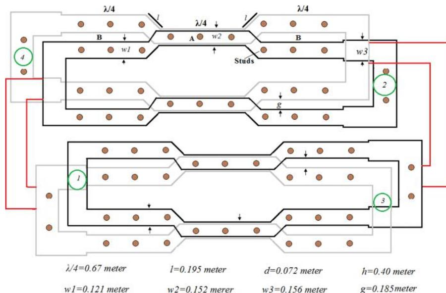
FIG. 7. Schematic of 1.5 MW, 3 dB hybrid coupler.
