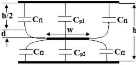
FIG. 3. Strip line with off-set rectangular strip.
