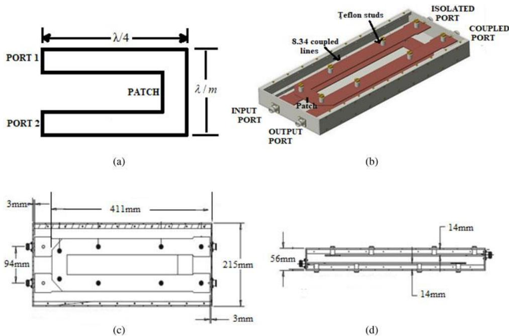
Fig. 4. Detailed assembly drawing of prototype tandem hybrid coupler. (a) U-shaped strip-line, (b) layout design, (c) top view, (d) side view of prototype coupler.
