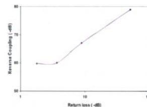
Fig. 5. Variation of return loss Vs reverse coupling at 13.56 MHz
