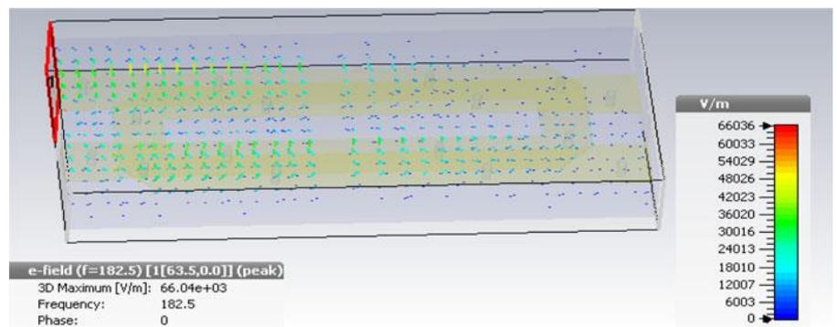
Fig. 6. Electric field plot of tandem hybrid coupler.
