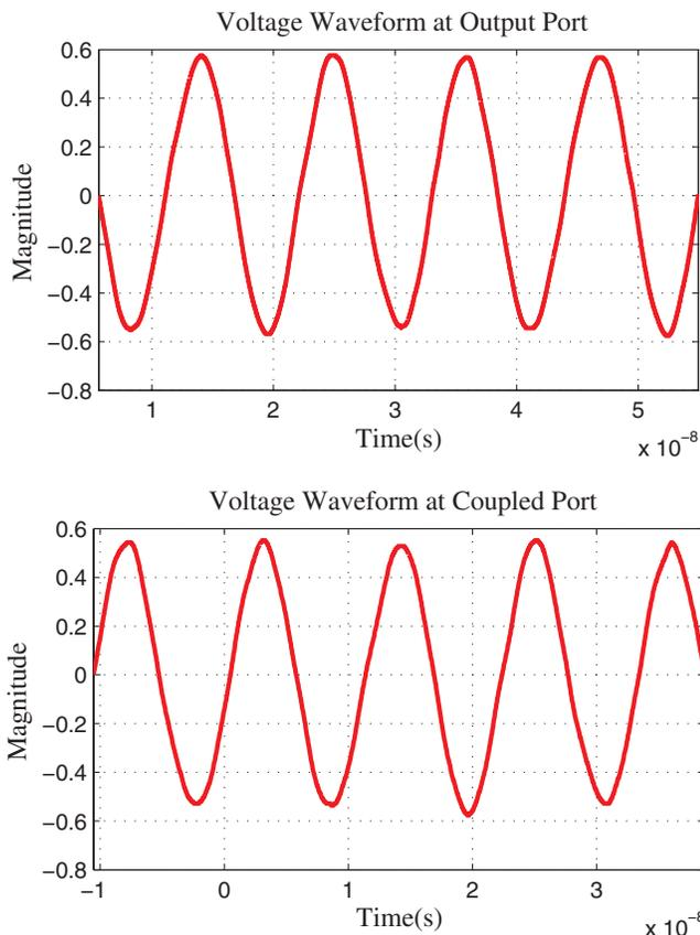
FIG. 12. Measured voltage waveforms at coupled and output port at 1.0 kW input.
