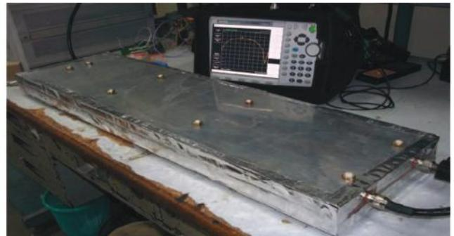
FIG. 9. Photograph of the fabricated hybrid coupler.
