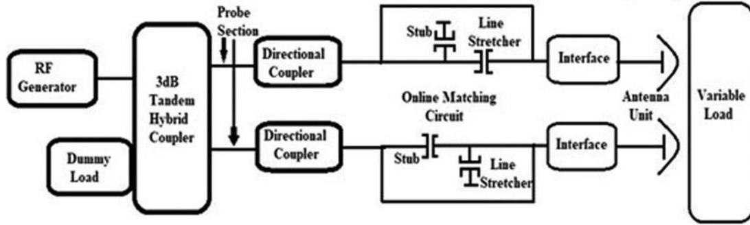
Fig. 1. Schematic representation of typical ICRF system.
