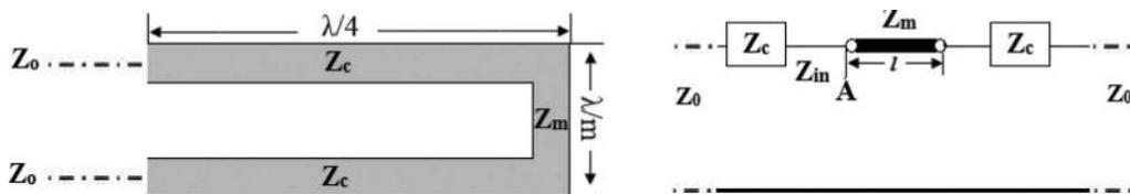
FIG. 6. U-shaped coupled strip line and equivalent circuit diagram.
