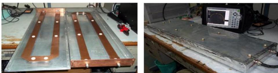
FIG. 2. Photograph of the inner assembly of the fabricated 2 kW, 3 dB tandem hybrid coupler.
