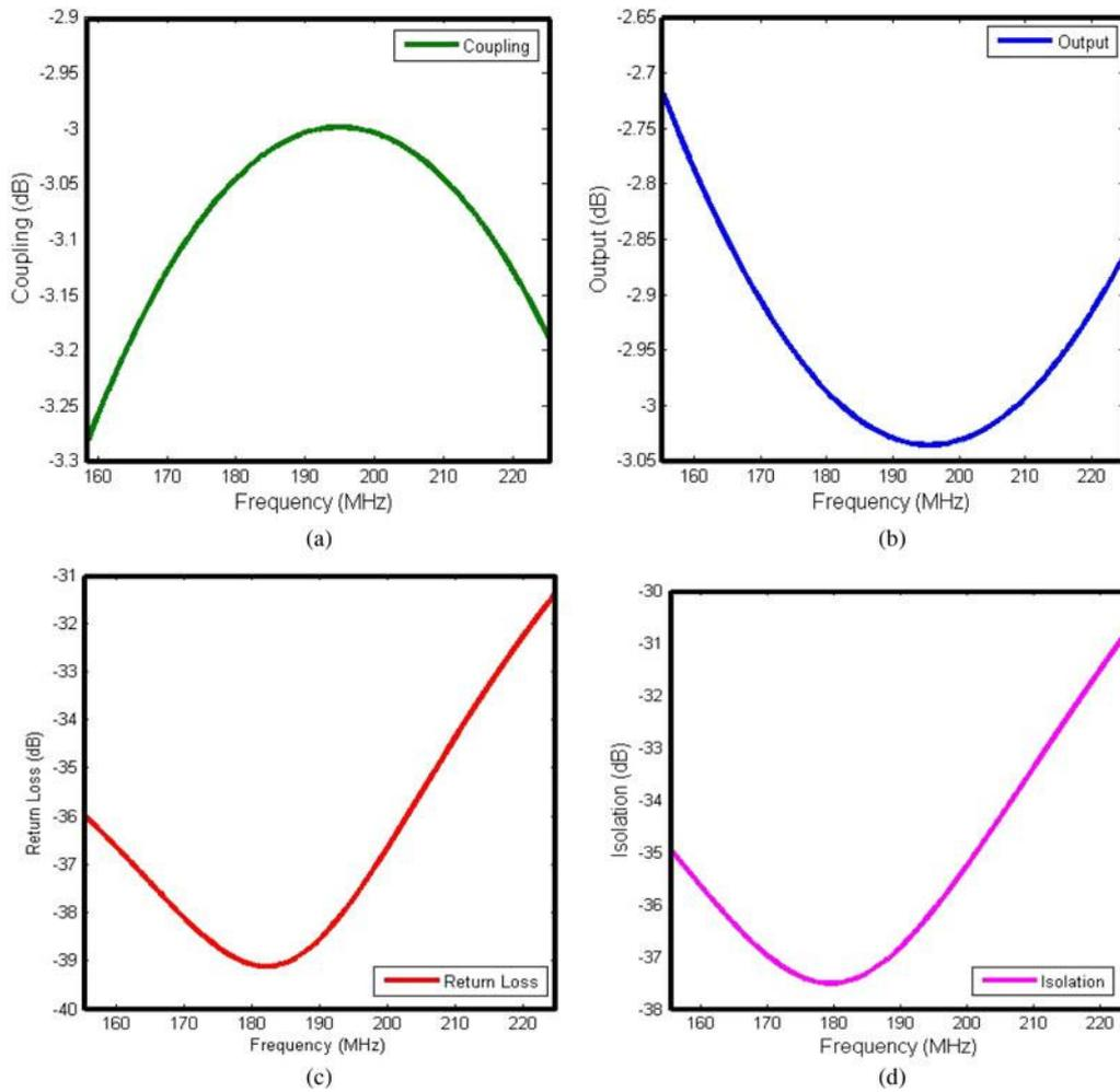
Fig. 5. Simulated S-parameters using CST software. (a) Coupling, (b) output, (c) return loss, and (d) isolation in dB.
