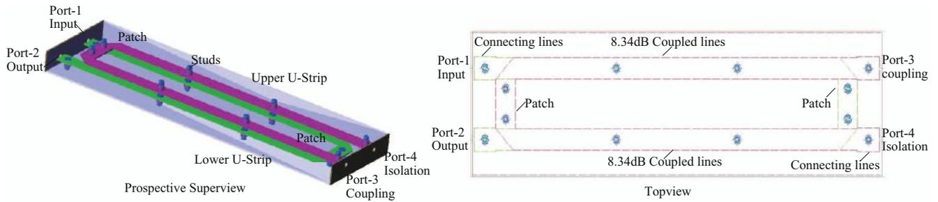
FIG. 1. Proposed tandem 3 dB hybrid coupler.
