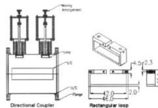
Fig. 1. Schematic of coaxial directional coupler.
