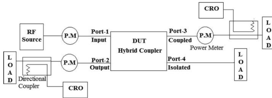
FIG. 11. Schematic diagram of high power test setup.
