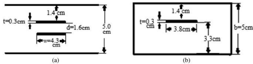
Fig. 3. Dimensions of coupled and patch section.
