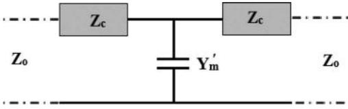
FIG. 7. Equivalent circuit diagram of strip line of tandem coupler.
