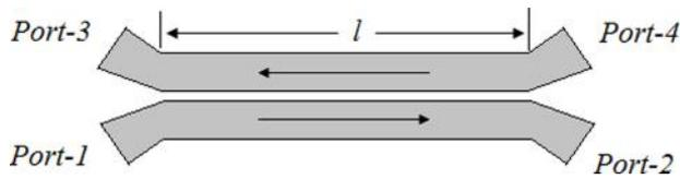
FIG. 1. Schematic of the 3 dB hybrid coupler.
