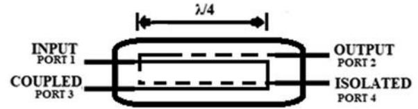
Fig. 2. Schematic representation of the 3 dB tandem hybrid coupler.
