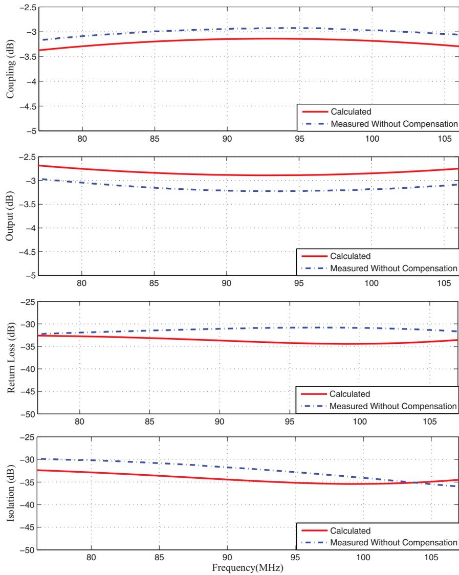
FIG. 5. HFSS optimized design results and the measured S-parameters without compensation.
