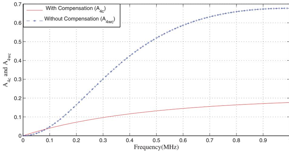
FIG. 8. Analytic comparison of isolation of compensated and uncompensated hybrid coupler.
