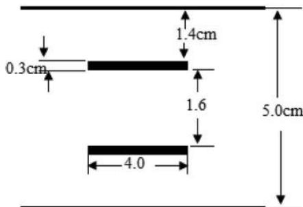
FIG. 4. Final dimension of the coupled and non-coupled line sections.
