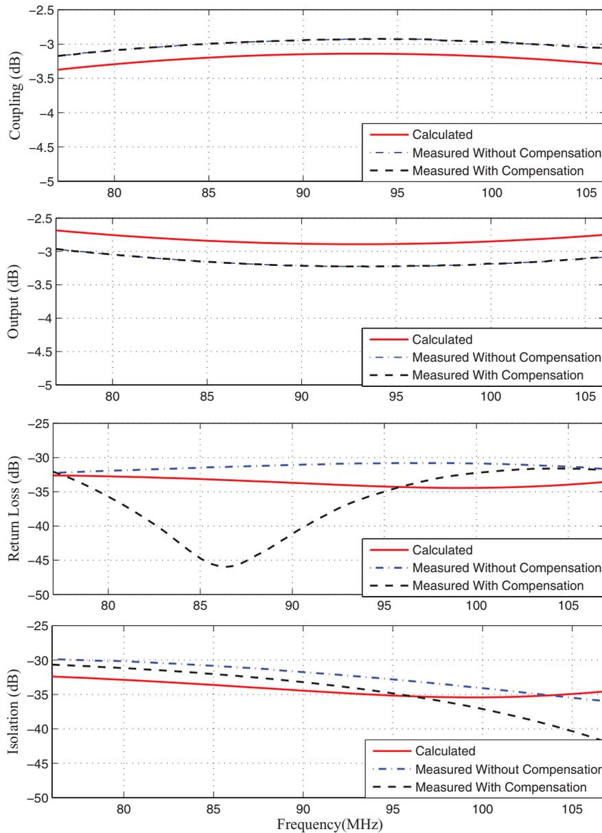
FIG. 10. Comparison of HFSS optimized design results, the measured S-parameters without compensation and with compensation.
