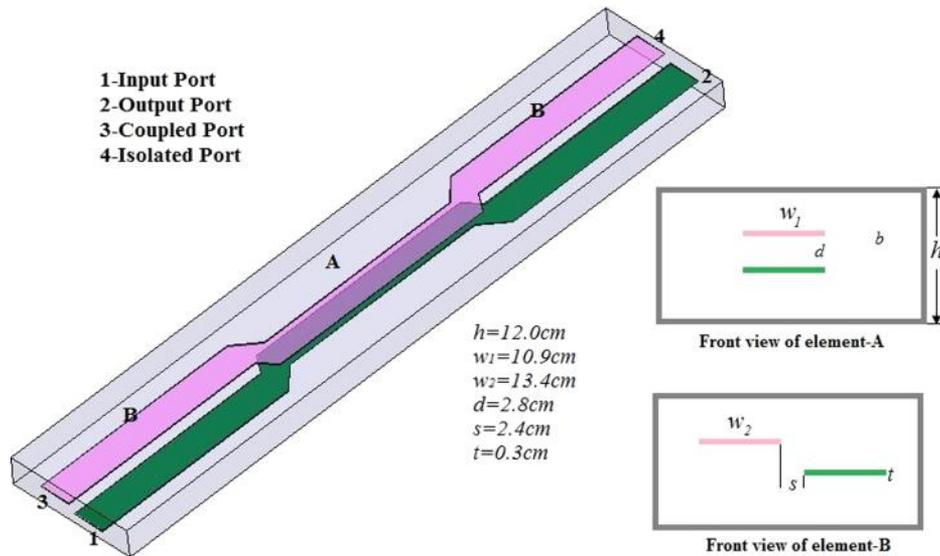
FIG. 3. The 3-D model of 3-elements (namely, A, B, C), 8.34 dB coupled lines section used in simulation.
