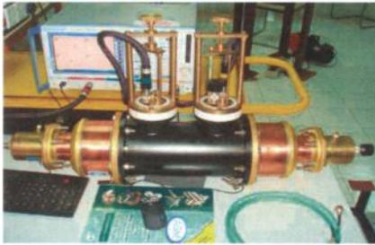
Fig. 2. Photograph of coaxial directional coupler.
