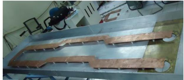
FIG. 4. Photograph of the inner one side assembly of the fabricated 200 kW, (38-116) MHz, tandem 3 dB hybrid coupler.
