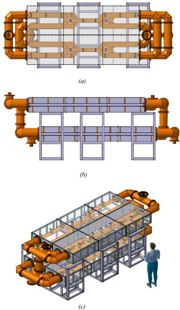
FIG. 9. Assembly drawing of the designed 1.5 MW 3 dB hybrid coupler. (a) Top view. (b) Side view. (c) Super view.
