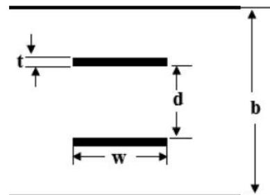
FIG. 2. Schematic diagram single 8.34 dB coupled strip line.
