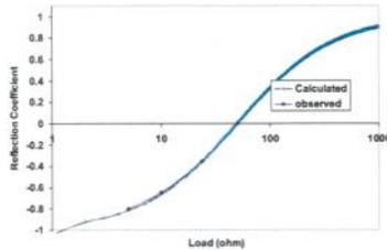
Fig. 7. Variation of load Vs reflection coefficient
