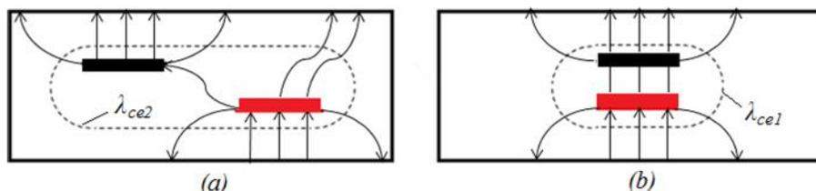
FIG. 6. Electric field lines for lowest TE modes in (a) Element-B and (b) Element-A.
