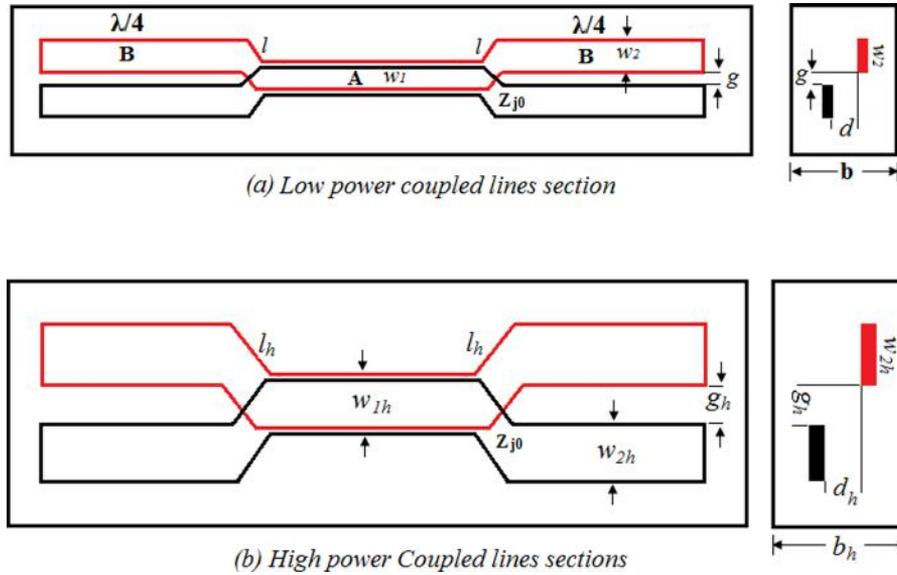
FIG. 5. Schematic of the (a) top and side view of low power, (b) top and side view for high power multi-element coupled lines.
