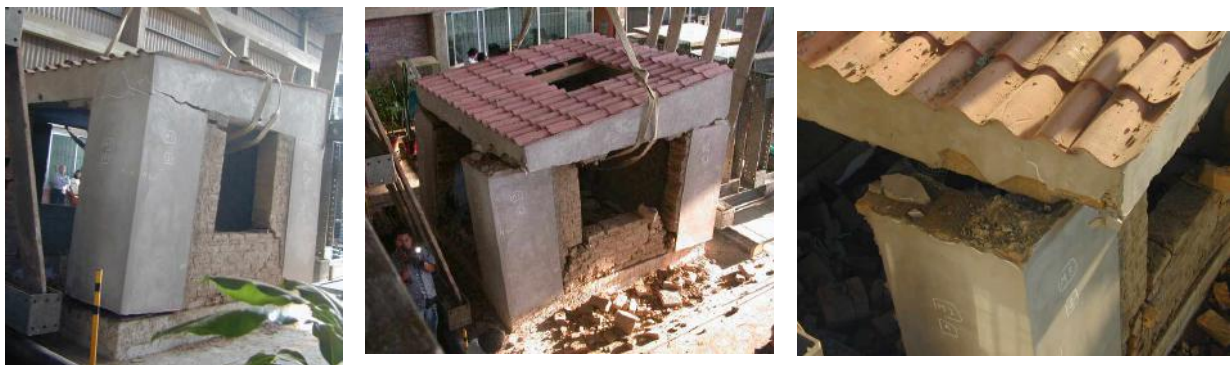
Fig. 8. Behavior of the module during the catastrophic earthquake simulation test (left), after the test (middle), and failure of the plain concrete shear key (right).
