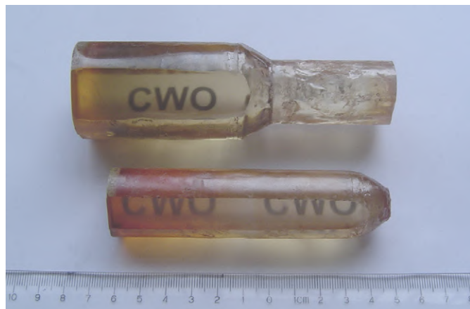
Fig. 2. CWO single crystal grown by vertical Bridgman process.
