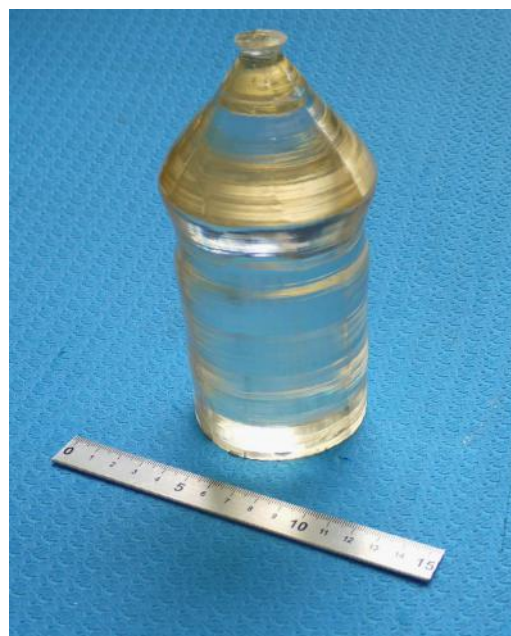
Fig. 2. The \text{CdWO}_4 crystals grown by LTG Cz method.
