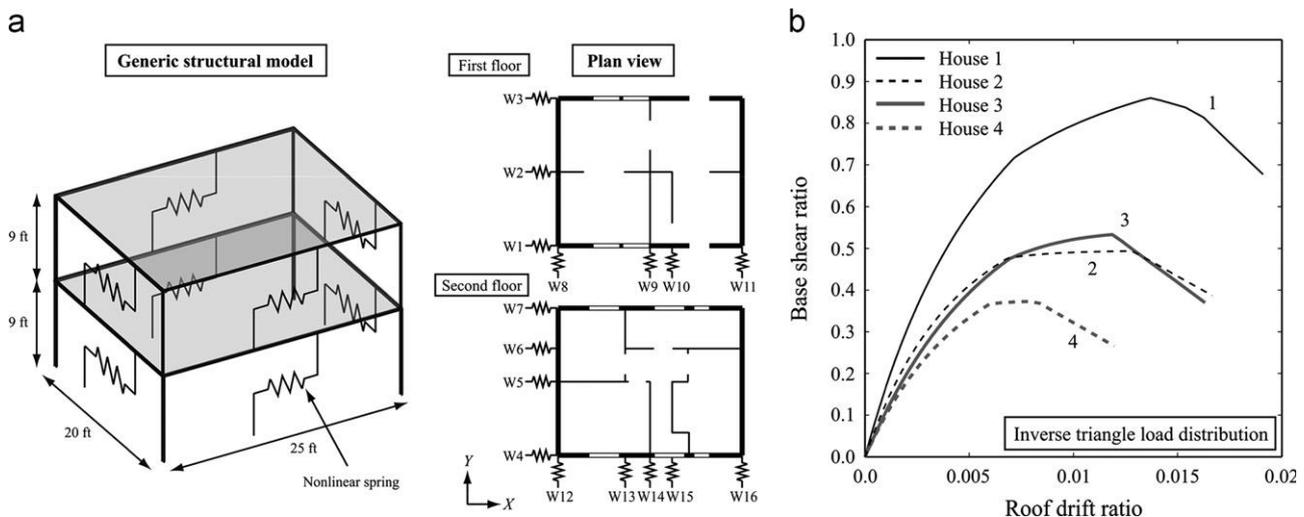
Fig. 1. UBC-SAWS model: (a) structural model and (b) static pushover curve.
