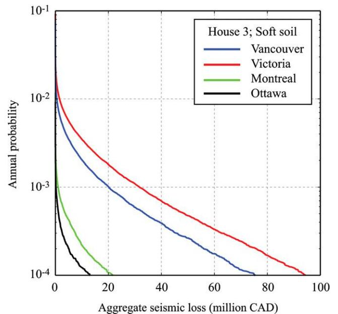
Fig. 13. Seismic loss curves for different locations (500 House 3; Soft soil; CMS-Event/Mag).
