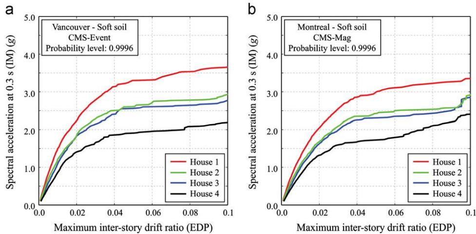
Fig. 12. Comparison of 0.50-fractile IDA curves for different house models: (a) Vancouver and (b) Montreal.
