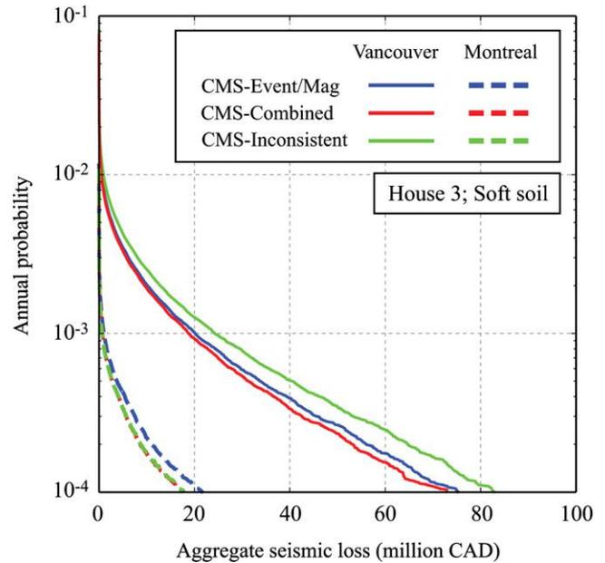
Fig. 15. Seismic loss curves for different IDA-CMS curves (Vancouver/Montreal; 500 House 3; Soft soil).
