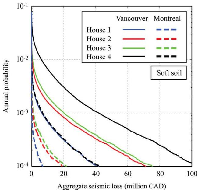
Fig. 16. Seismic loss curves for different house models (Vancouver/Montreal; Soft soil; CMS-Event/Mag).
