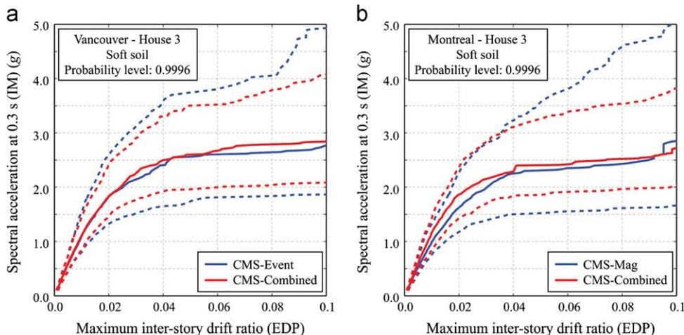
Fig. 11. Comparison of IDA curves for different CMS-based approaches: (a) Vancouver and (b) Montreal. The solid line corresponds to a 0.50-fractile IDA curve, while the broken lines correspond to 0.16- and 0.84-fractile IDA curves.
