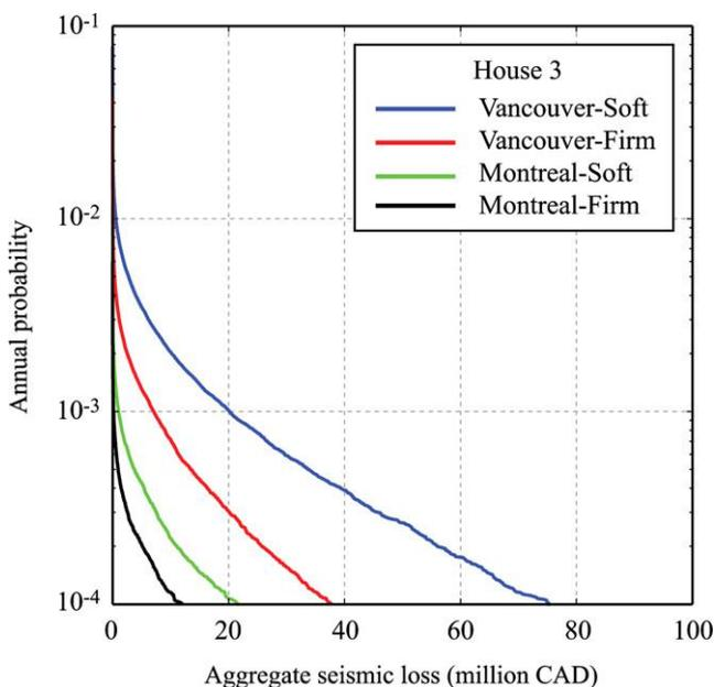
Fig. 14. Seismic loss curves for different site conditions (Vancouver/Montreal; 500 House 3; CMS-Event/Mag).
