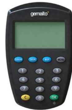
Fig. 5. A USB smart card reader with its own display and keypad.
