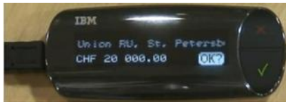
Fig. 8. IBM's ZTIC used to verify a transaction.
