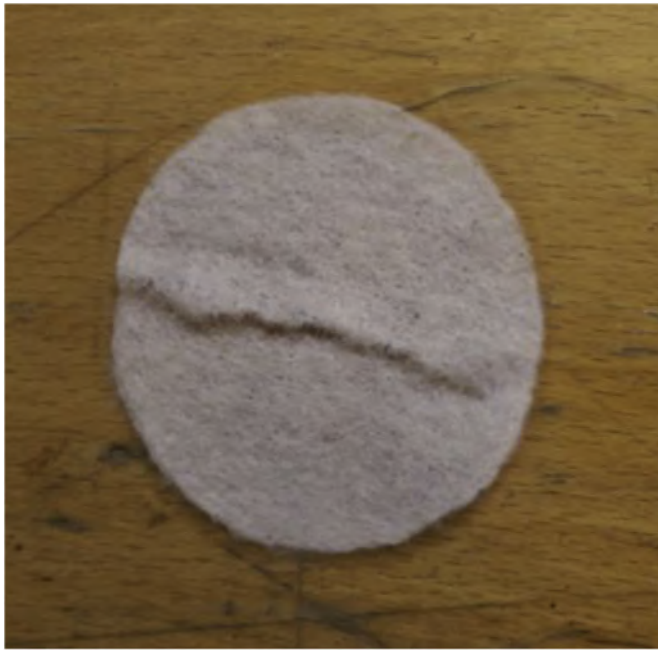
Fig. 12. Image of ruptured geotextile type 1 after experiment of samples with 94% relative density.
