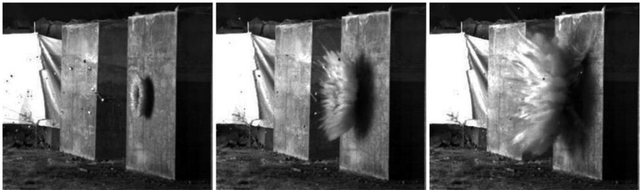
(a) The perforation progress of initial cratering
