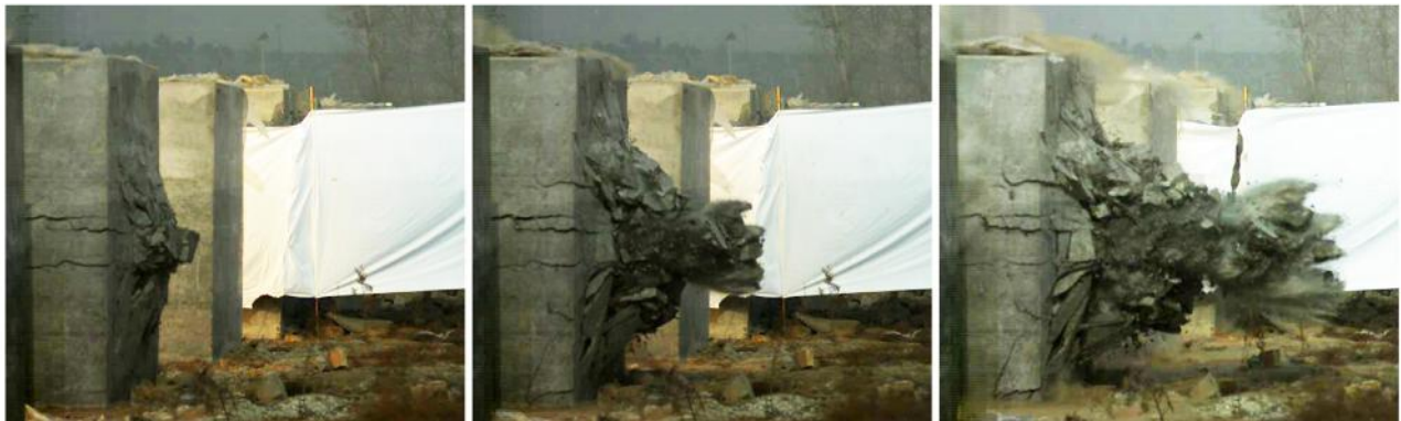
(b) The perforation progress of shear plugging
