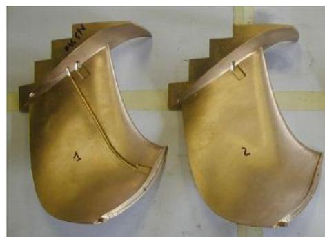
**Figure 12** Francis runner blades equipped with strain gages
