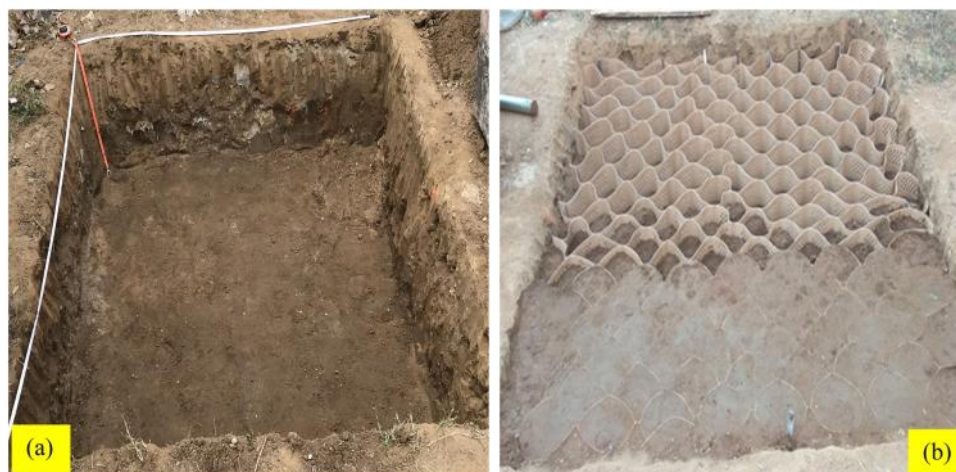
Fig. 5. Preparation of foundation bed: (a) excavated test pit; (b) partially filled geocell reinforcement.
